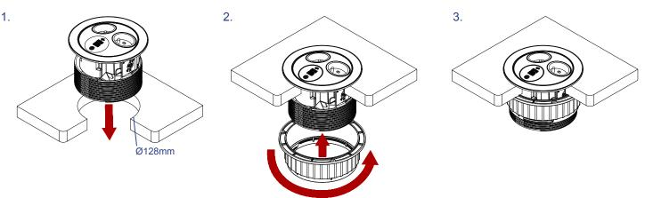
pandorARC drops into a 128mm<sup>+</sup> grommet hole e.g. in a table top and is then secured by tightening by hand the moulded securing nut. No tools are needed once the grommet hole is cut, but access below/behind the fixing surface is required.
